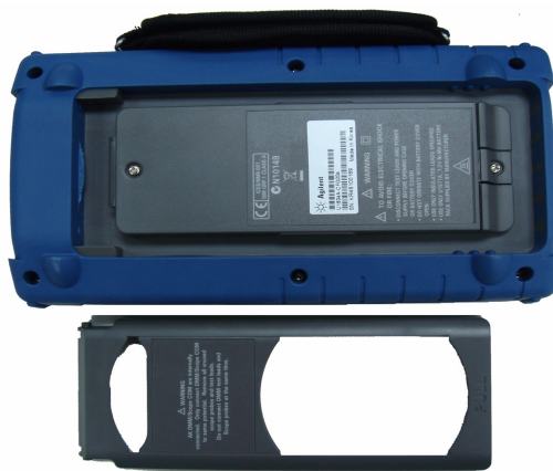
Figure 8-2 Disassemble the stand from the instrument
