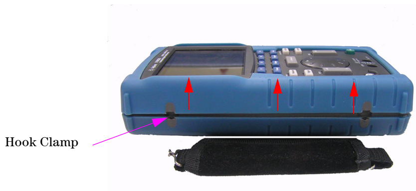
Figure 8-8 Remove handler from the instrument
