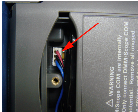
Figure 8-6 Unplug 2-wire connector with a tweezers.
