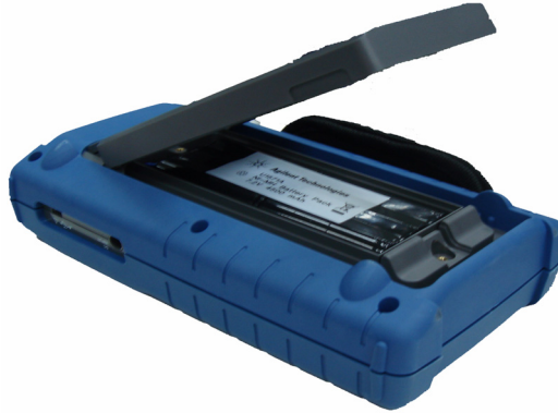
Figure 8-5 Remove battery pack cover without removing stand
