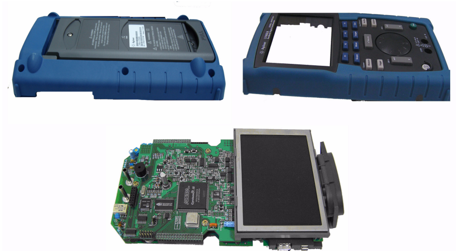
Figure 8-10 Remove front casing (right) and rear casing (left) from PCBA of the instrument
