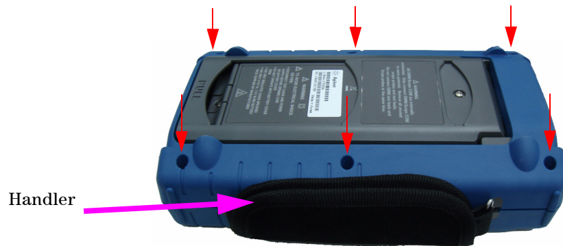
Figure 8-7 Remove screw from the rear cover
