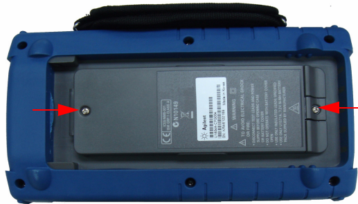
Figure 8-3 Remove battery cover screw
